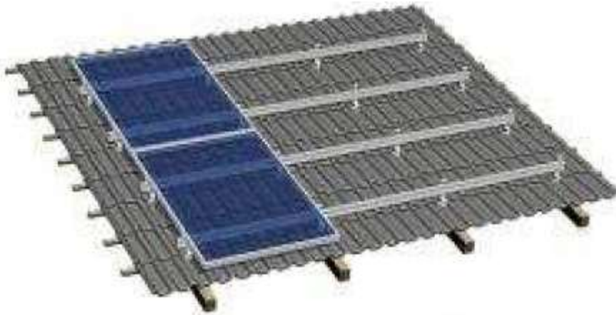
Figure 1 - Typical Mounting system on rooftop
